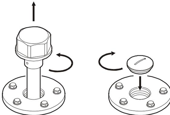
Figure 19: Complete Removal of Fuel Level Sensor
