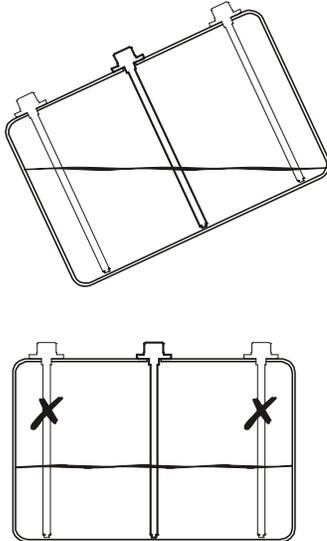
Figure 2: Correct Position of Sensor on Fuel Tank
