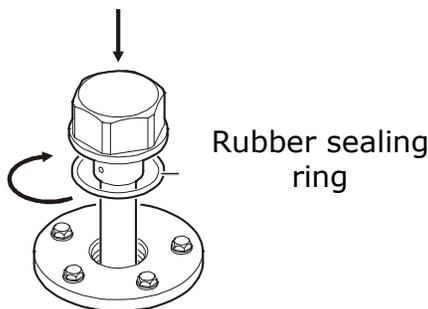
Figure 7: Installation of Assembled Sensor on Fuel Tank
