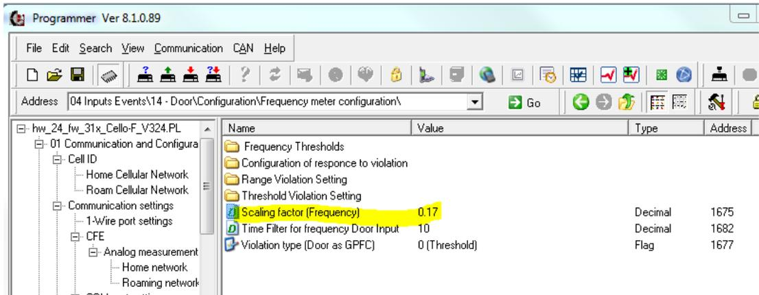
Note that since the maximum frequency value is 1500 Hz and the maximum value represented in a byte is 255, the scaling factor is  $255/1500=0.17$
