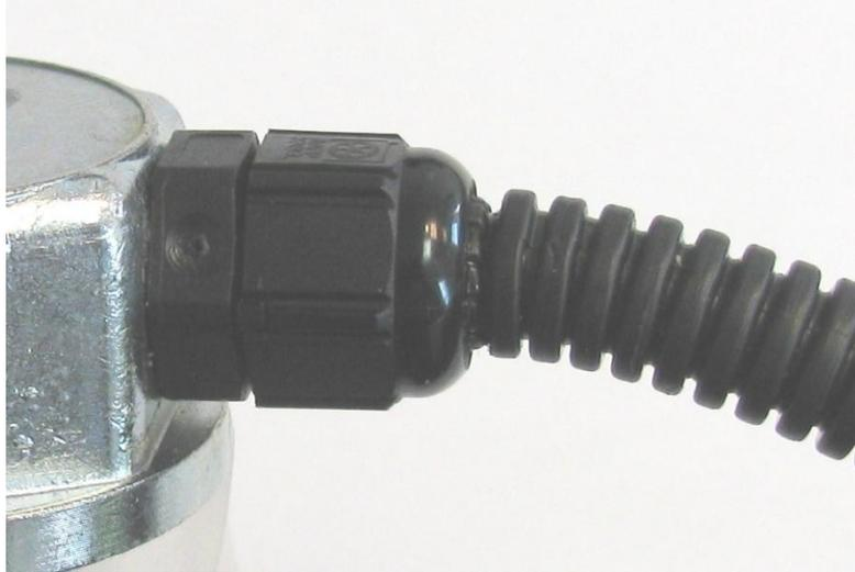
**WARNING:** Do not twist the cable entry on the measuring head; this may violate the integrity of the sealing and electrical connectivity between the measuring head and the interface cable.
