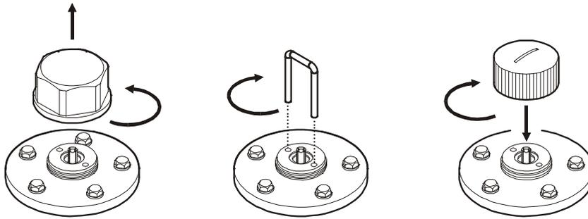
Figure 18: Removal of the Measuring Head
