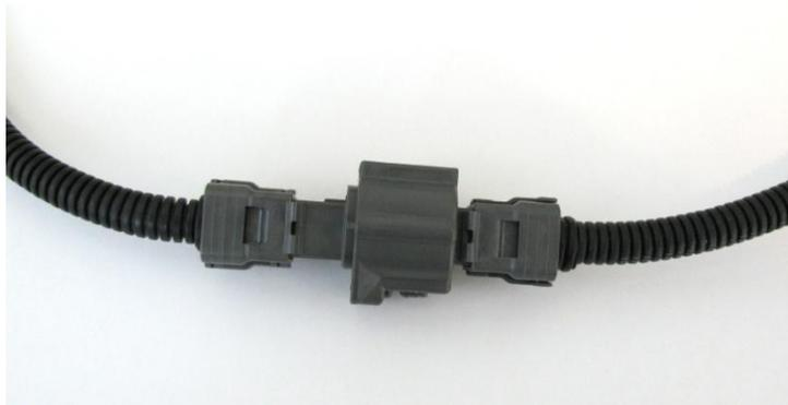
3. The fuel sensor harness should be installed from the sensor which is installed on the fuel tank, to the Cellocator unit, which is usually located in the driver's cab, through the holes provided within the vehicle structure. The harness should be fixed with cable ties on immovable parts of the structure every 50-60 cm.
