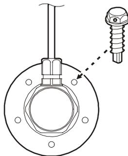
Figure 4: Position of Screw with a Hole for Sealing
