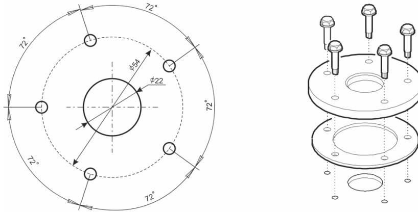
Figure 3: Size and Method of Flange Setting on Fuel Tank
