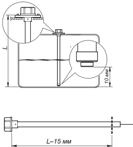
Figure 5: Measuring Probe's Length
