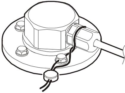
Figure 8: Sealing the Installed Fuel Level Sensor
